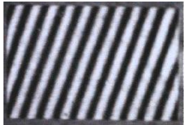
Figure 1 Interferogram of a very flat surface ...straight, parallel fringes.
